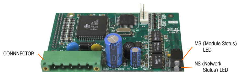
Figure 3-2: DeviceNet Option Board Components
