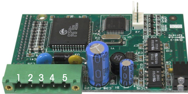
Figure 3-3: DeviceNet Connector Pin Numbering
