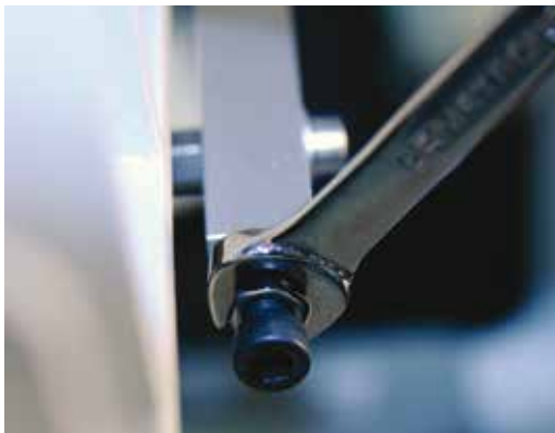
Figure A4: Loosen the lock nut
