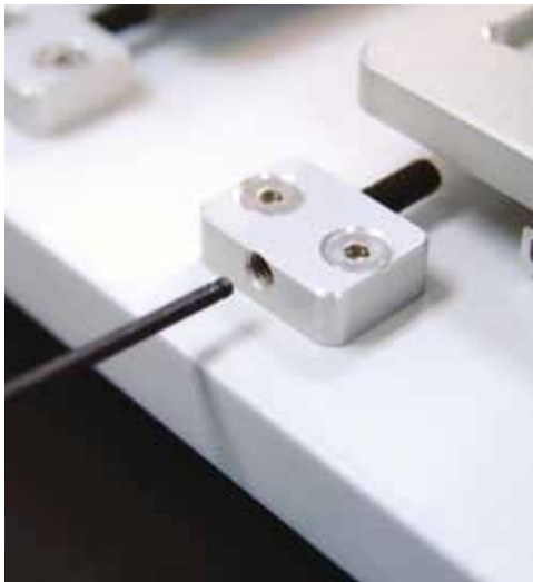
Figure A8: Hex driver engaging front tray stop screw
