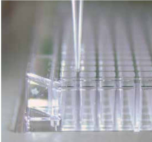
Figure A10: Proper location of tip between the four wells in the left corner of the plate
