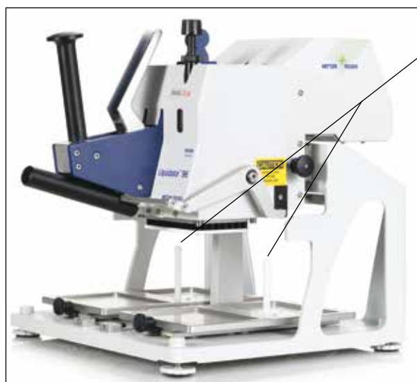
ADJUSTMENT SCREWS AT ENDS OF POSTS
