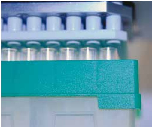
Figure A3: Non-aligned nozzles (exaggerated view)
