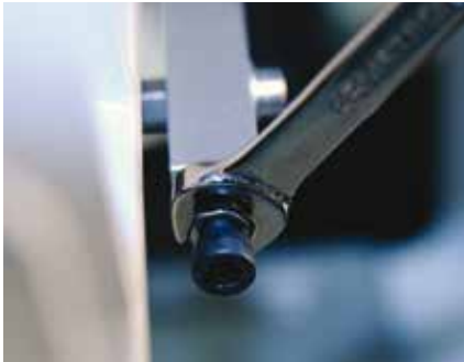
Figure A5: Adjusting the right stop
