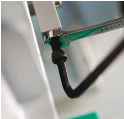
Figure A6: Tightening the lock nut
